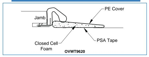
Loxcreen's new and improved corner pad is the perfect complement to our 9650 MPC foam weatherstrip. Our corner pad features a new high performance cover and closed cell foam core that provides maximum prevention of air and water infiltration.
